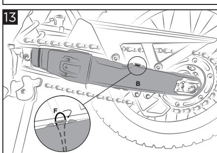
**Mount the fork protection (B) framing it with the support (D) and hook the rubber band (F).**
