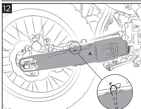
**Mount the fork protection (A) framing it with the support (C) and hook the rubber band (F).**
