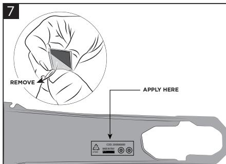
**Clean perfectly the swingarm and the teket magnet protection removing any trace of dirt, grease and oils in the indicated area. Remove the biadhesive's protective film (H) from one side and paste it on the inside of the protection (A)/(B), as shown in figure (above the plastic details panel).**
