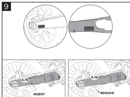
**Place the swingarm protections (A)/(B) and applying pressure in the fixing areas of the velcro and remove it, checking that the velcros are placed correctly on the protection and the swingarm.**
